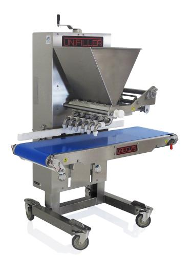
Traditional confectionary gearwheel depositors are used worldwide, and are known for performing very well but with limitations in production speed and type of products. In these applications the UNI-FILLER Multi Stations M600 and M800 are the perfect solution to traditional gearwheel confectionary depositors.
